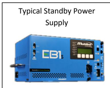
When a utility power outage occurs the standby power supply automatically switches to a battery backup mode and keeps the network operating for a relative short period of time. Perhaps 2 hours more or less depending on number of batteries and the load. When the power supply switches to battery backup mode an alarm is sent to the management system giving notice of the event and triggers a plan of action should the outage persist.
